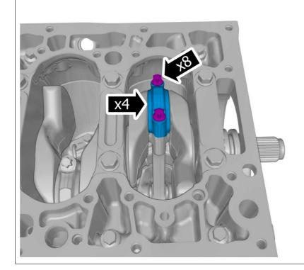
Warning! Make sure that new bolts are installed.
