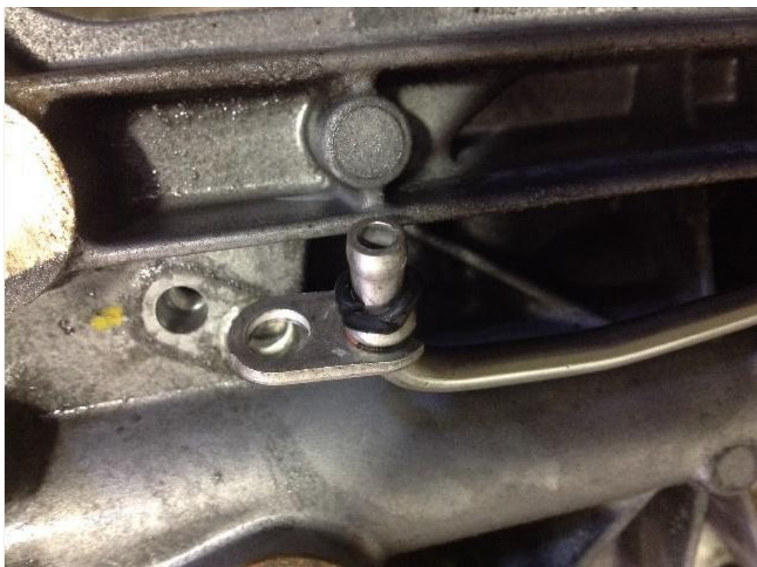
Vacuum connection on mounting plate.JPG:
