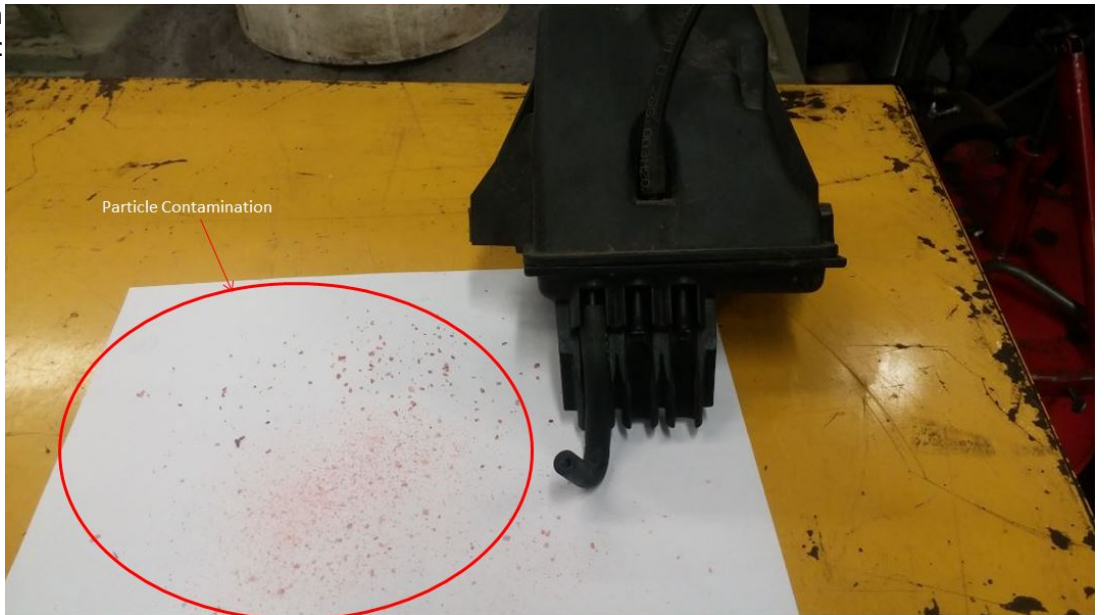
Particulate contamination of vacuum reservoir.JPG:
