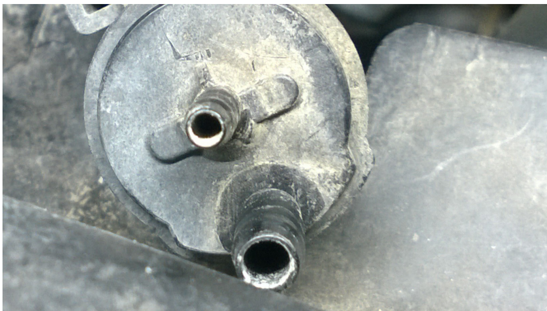
Contaminated EV Valve. jpg:
