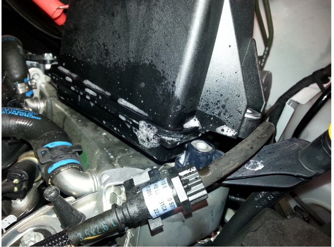
Leaking vaccum manifold.jpg:
