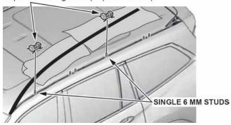
3. Install the two M6 clips (natural color) in the same location as the the original clips (the single 6 mm studs).
