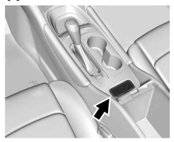
Wireless inductive charging uses an electromagnetic field to transfer energy between two objects. The wireless inductive charging system charging pocket is located just in front of and below the armrest of the center console. The operating temperature range for the charging system is between  $-4^{\circ}F$  ( $-20^{\circ}C$ ) and  $140^{\circ}F$  ( $60^{\circ}C$ ) and for the mobile device between  $32^{\circ}F$  ( $0^{\circ}C$ ) and  $95^{\circ}F$  ( $35^{\circ}C$ ).
