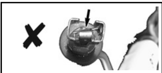
TERMINAL OUT OF FUSE BOX - DEFORMED
