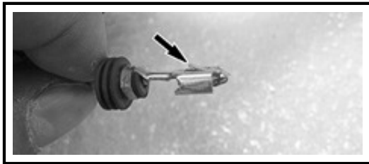
TERMINAL LOCKING TAB EXCEEDING
