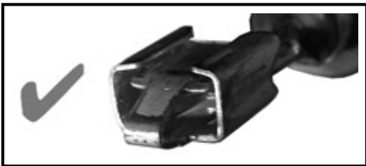
TERMINAL OUT OF FUSE BOX - GOOD
