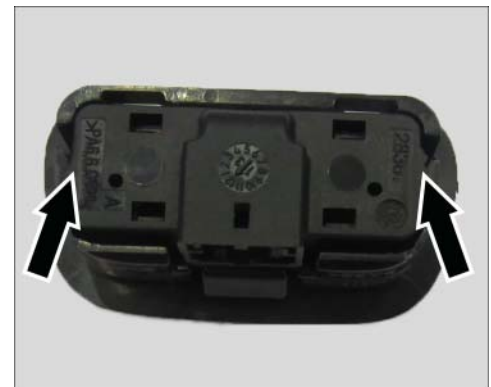
Affixing fuel tank readiness switch in trim surround
