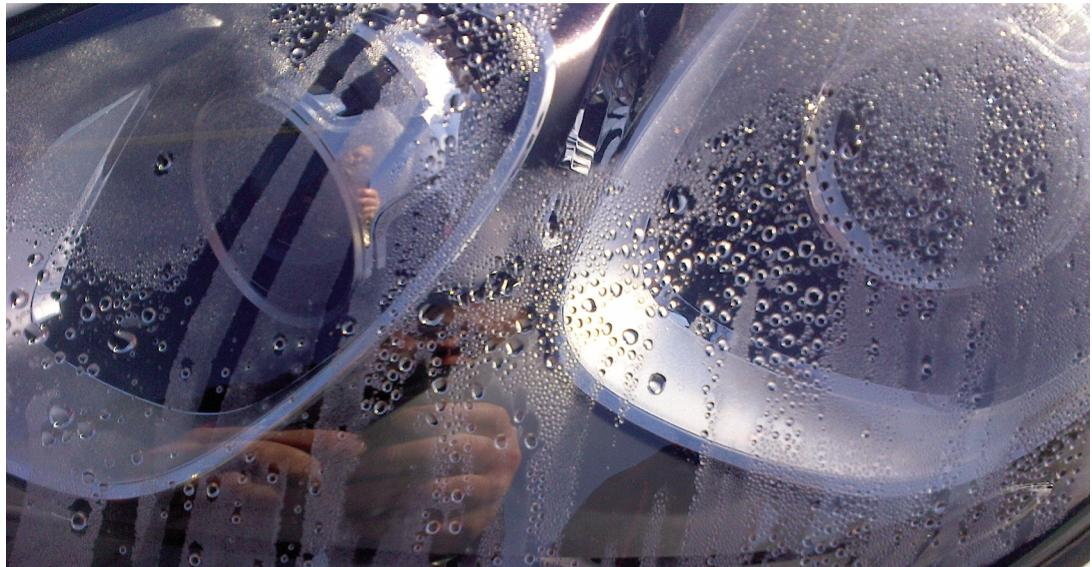
In the event of excessive moisture buildup, inspect the headlamp for leaks around the lens. If no leaks are present, inadequate ventilation of the headlamp is not allowing the moisture to escape.
