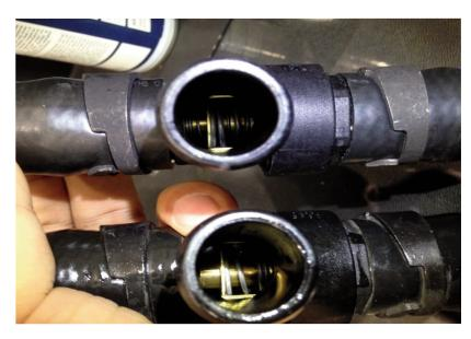
Replace the coolant hose with the built in thermostat if any of the above listed faults are stored in the power electronics. If additional technical support is required, submit a PTEC-TLAR.
