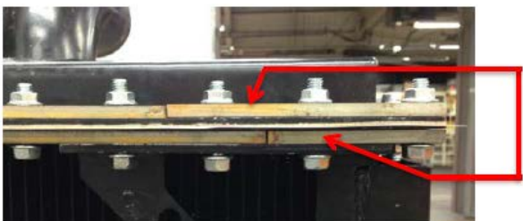
C-Shaped Bars and Staggered Seams
