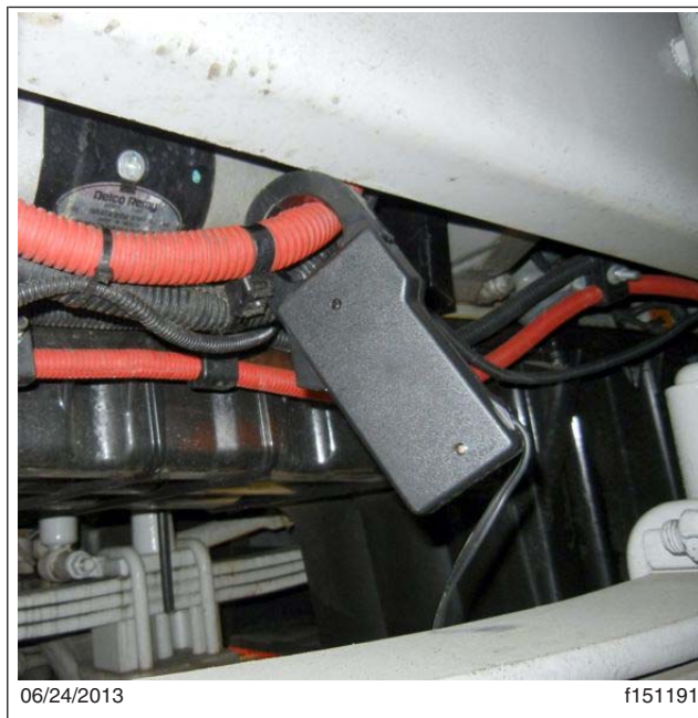
Fig. 9, Measure the crank amperage with an amp clamp on the positive starter cable during crank.
