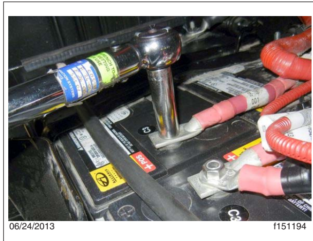
Fig. 11, Check the battery connections for looseness and corrosion. Check the torque on the connections.
