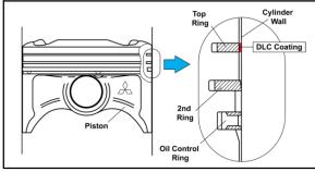
b. New top piston ring contact surface has Diamond Like Carbon (DLC) coating to reduce friction.
