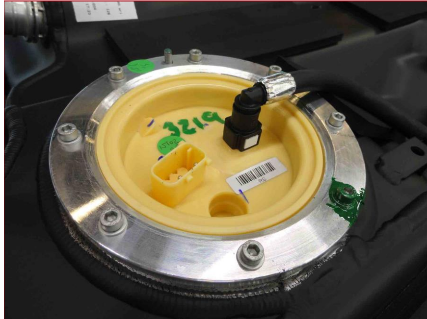
Pompa/e carburante Fuel pump/s
