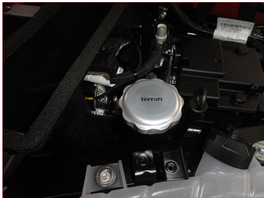
Serbatoio olio Oil tank
