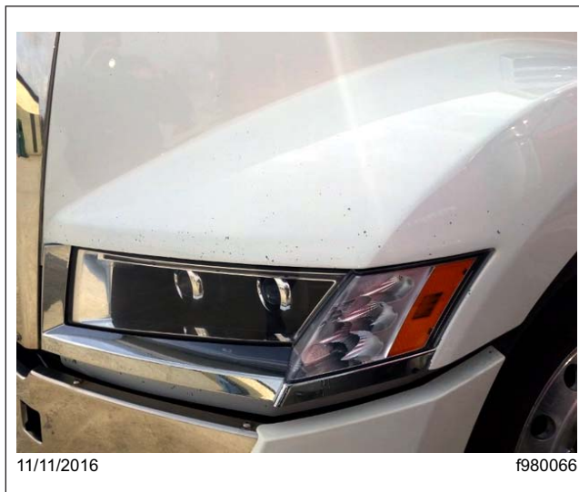
Fig. 1, Chipped Paint from Road Debris
