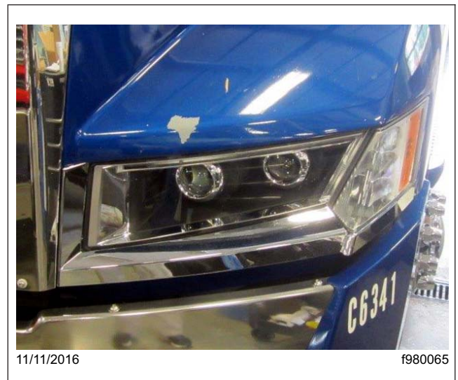
Fig. 2, Paint Does Not Adhere to the Hood
