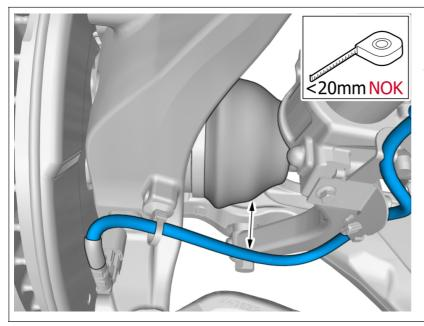
If the distance is less than 20mm, the wiring needs to be repositioned according to the following steps.
