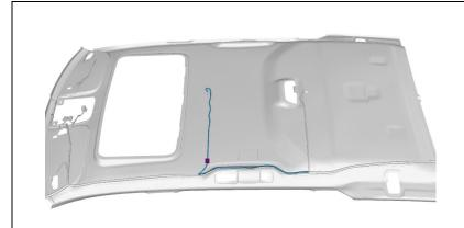
Route the cable to rear sensor and connect the adapter cable
