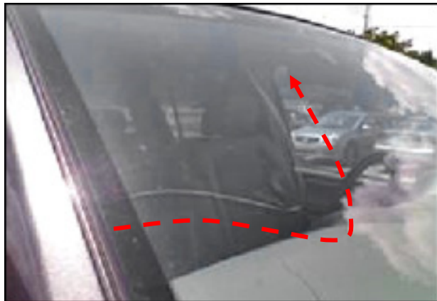
Single crack with no impact mark: Warranty
