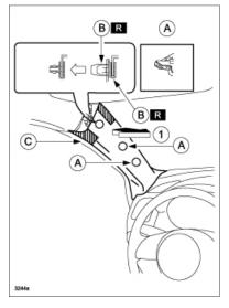
Grommet (B) for Lead Wire (A) by A-pillar trim (C)
