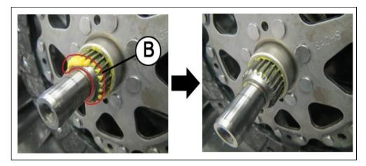
4. Slide the clutch disc a few times to spread the grease.
