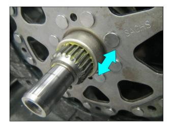
5. Remove the clutch disc from the main drive gear shaft and remove excess grease (C).
