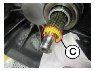
6. Install the clutch assembly. Refer to MS3 Workshop Manual CLUTCH UNIT REMOVAL/INSTALLATION. No additional grease to the spline is needed when installing the clutch unit.
