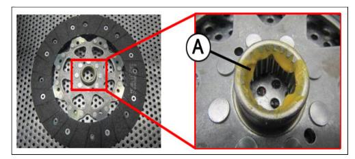
3. Insert the clutch disc to the main drive gear shaft and remove excessive grease (B).
