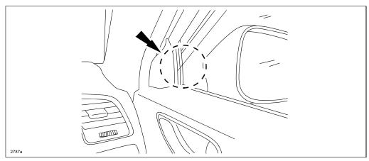
The rattle noise may be caused by insufficient holding force of the glass run channel. To increase the holding force, the shape of glass run channel has been changed and non-woven pads have been attached to the glass run channel.
