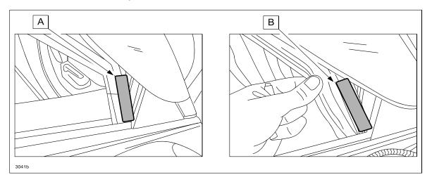
6. Apply an adhesion promoter (one that is suitable for use on plastic) to the locations where the pads will be attached.
