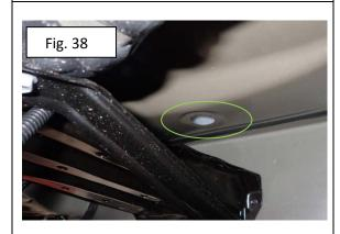
29. Make a cut in the center of body plug by folding and using side cuts or equivalent to make an incision in center of plug.
