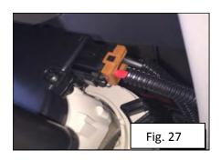
14. Tilt vacuum inward and disconnect the electrical connector.
