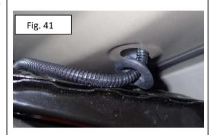
32. Locate the harness in the driver's floor pan under carpet. Pull harness into vehicle.
