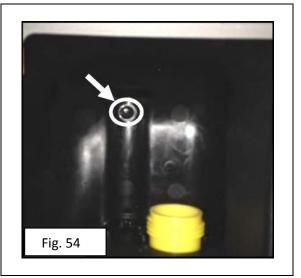
43. Install hose assembly by threading nut on hose end onto hose attachment point inside hose storage cavity. Press power button again to test vacuum air path connections - suction should be felt at end of hose assembly. Turn vacuum off using power button.
