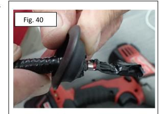
31. Push Harness into body through body plug hole.
