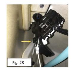
16. Remove the wire retainer on the back of the harness power connector by prying clips away from housing body and sliding back.
