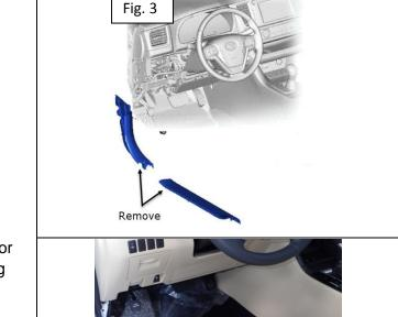
2. Pull carpeting away from floor board in area behind parking brake pedal.
