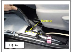
33. Route Harness with factory harness along left side of vehicle to rear quarter on board vacuum location.
