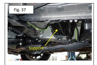
28. Locate and temporarily remove floor pan plug above support.
