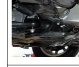
26. Route harness down back of wheel well and to the inside of the body seam.
