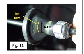
17. Route accessory wiring harness through grommet. One Terminal at a time.
