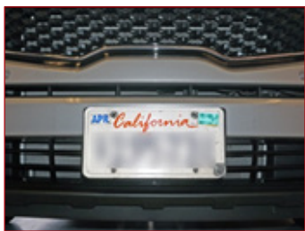
Radar module partially blocked: plate mounted incorrectly
