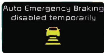
Radar module partially blocked: plate mounted incorrectly
