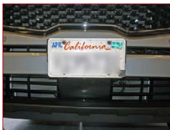
Radar module unobstructed: plate mounted correctly
