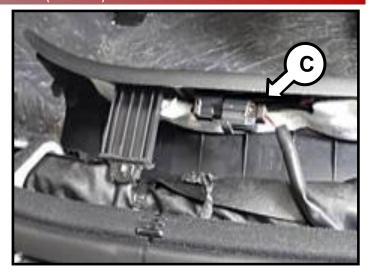
Remove the hood latch release handle
