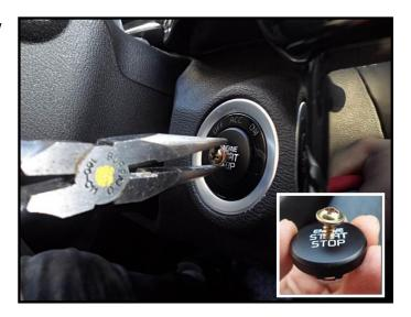
4. Inspect the SSB cap for damage to the cap hooks (B).
