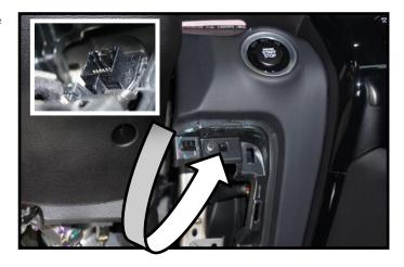
11. Press the release button on the top middle of the connector and pull connector out.
