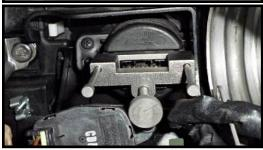
14. Press center plunger to eject the SSB assembly from the dash panel.
