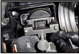
13. Engage the release fork to release the anchoring tabs of the switch.
