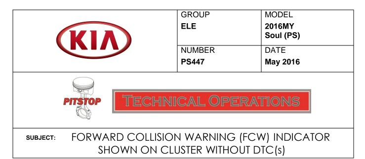
On some 2016MY Soul (PS) vehicles, you may see a Forward Collision Warning (FCW) indicator may appear on the instrument cluster with no DTC's present. This condition may be caused by incorrect/lost variant coding of the Lane Departure Warning System (LDWS) camera, or when replacing with a new camera. Follow the procedure outlined below to resolve the concern
