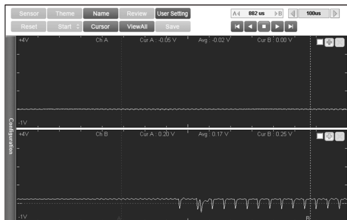
High Shorted to Ground - High at Zero
