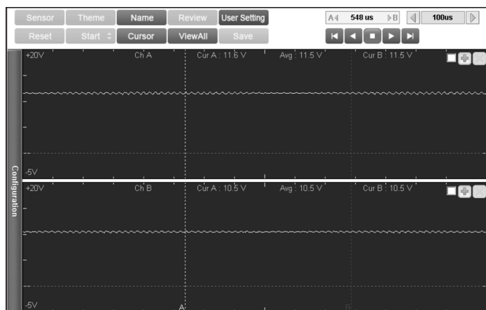
High Shorted to Power - High at B+
