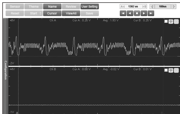
Low Shorted to Ground - Low at Zero
