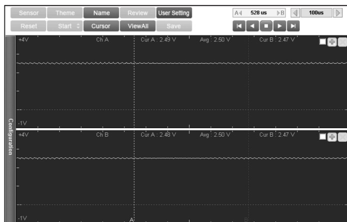
High and Low Lines Shorted Together
