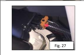
14. Tilt vacuum inward and disconnect the electrical connector.
