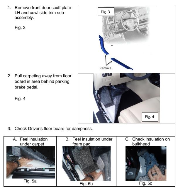
**Note**: If uncertain of water intrusion, perform water leak test while monitoring the area behind the parking brake in the area of the hood release cable grommet.
