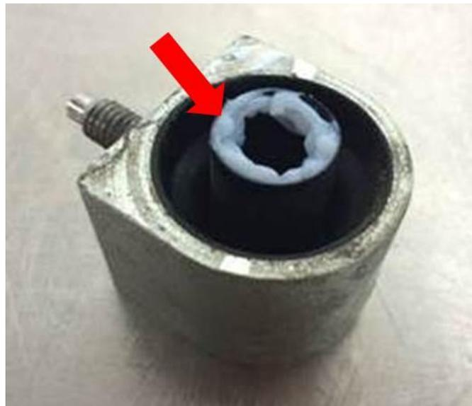
**Fig. 6 Bushing Greased**
