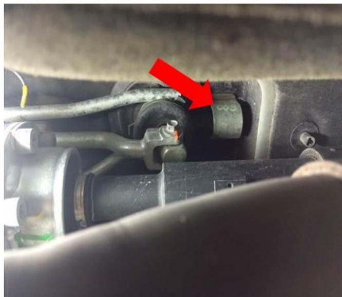
**Fig. 4 Bushing On Shifter Rod**
