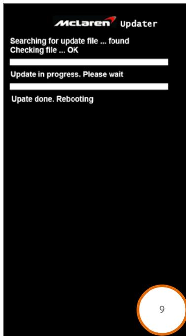
48. Following the reboot the system will start to update the individual system components (10), (11). During the update the system may reboot multiple times. This is normal, **do not attempt a manual reset**.
