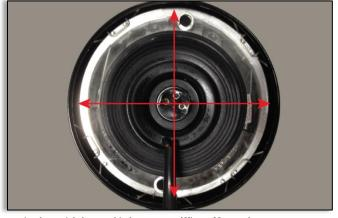
9. On the front of the bezel make sure the lens and bezel are properly aligned as shown.
