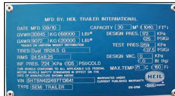
Figure 1. Example Identification Plate
