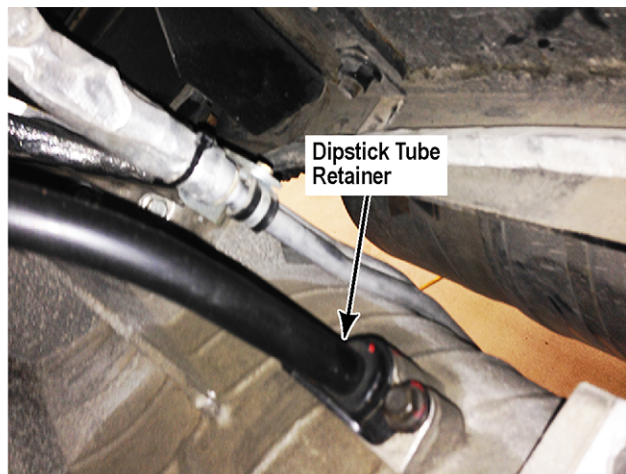
Dipstick tube and retainer (view from top)
