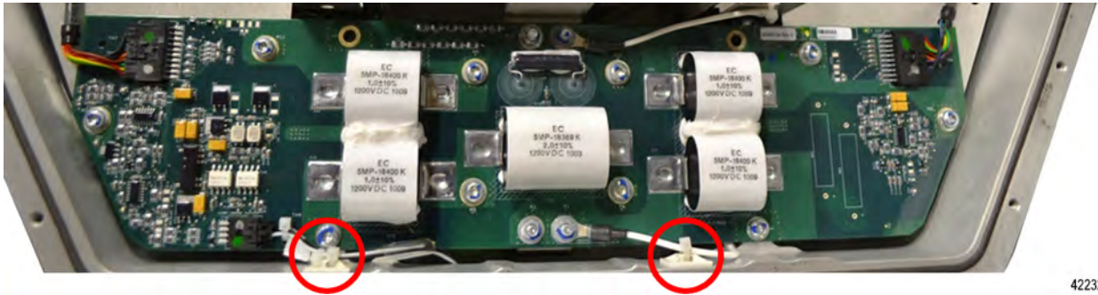
Figure 8. HVIL Circuit Card – Two (2) Wire Tie Locations
