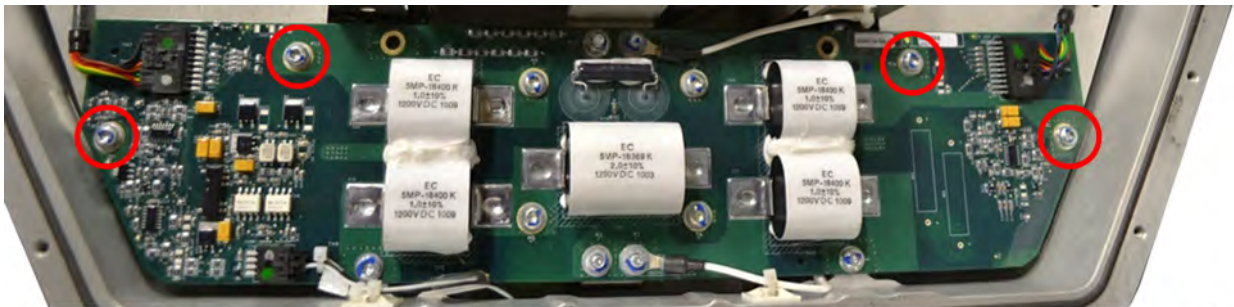
Figure 14. HVIL Circuit Card – Four (4) Mounting Screw Locations (M5x22mm)
