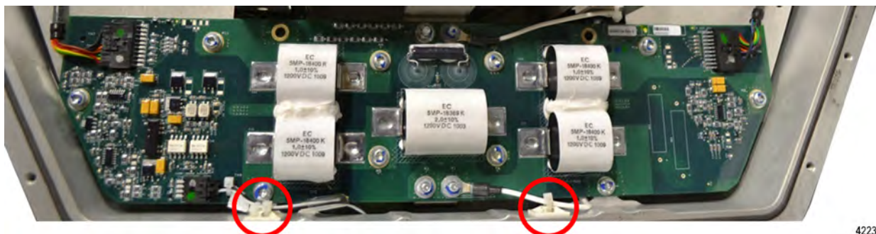
Figure 25. HVIL Circuit Card – Two (2) Wire Tie Locations
