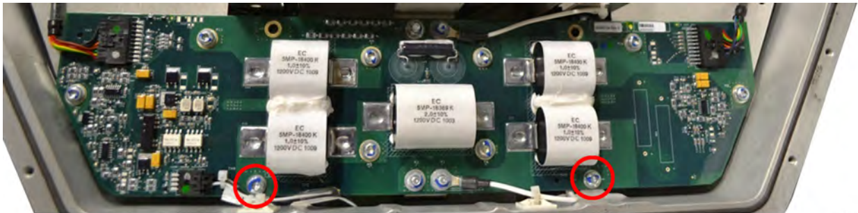
Figure 13. HVIL Circuit Card – Two (2) Mounting Screw Locations (M5x14mm)
