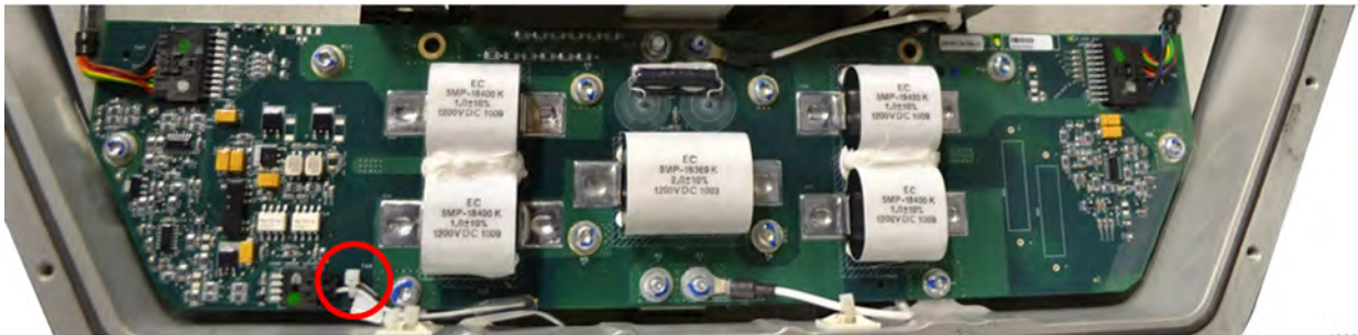
Figure 7. HVIL Circuit Card – Wire Tie Location
