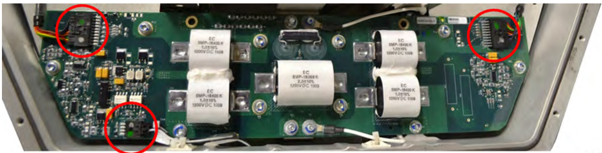
Figure 22. HVIL Circuit Card – Three (3) Harness Connector Locations
