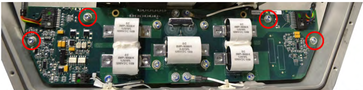
Figure 15. HVIL Circuit Card – Four (4) Mounting Screw Locations (M5x22mm)
