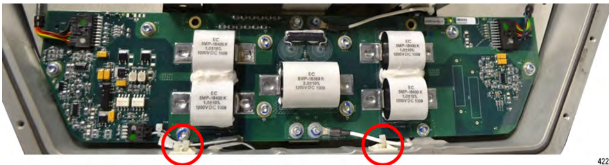
Figure 9. HVIL Circuit Card – Two (2) Wire Tie Locations
