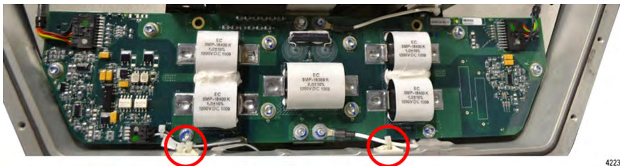
Figure 51. HVIL Circuit Card – Two (2) Wire Tie Locations
