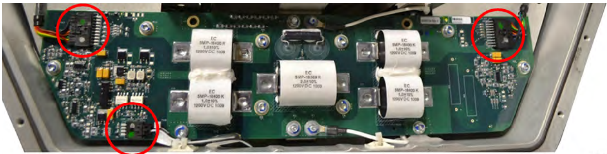
Figure 48. HVIL Circuit Card – Three (3) Harness Connector Locations
