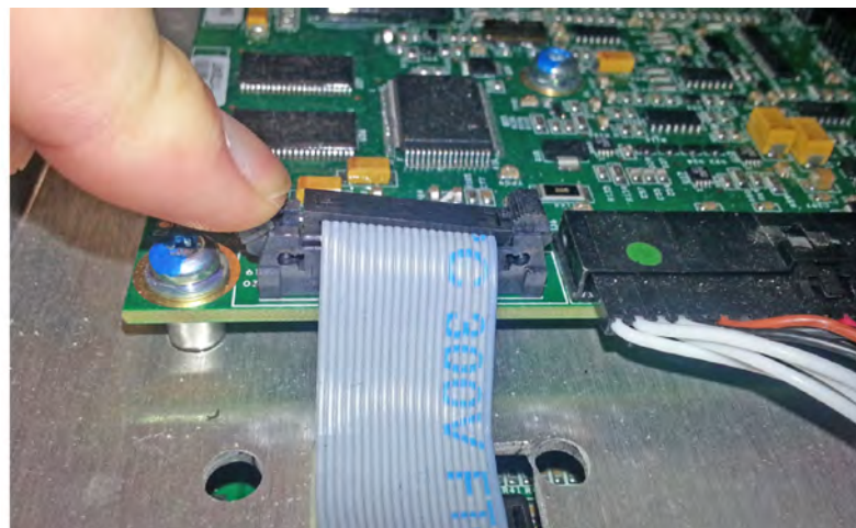
Figure 41. GATE Drive Card Cable Connector Installation (BCA Card Cable Connector Shown for Clarity)
