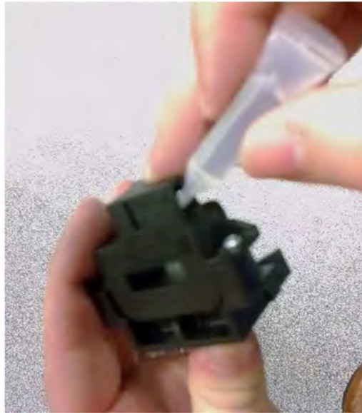
Figure 35. Applying NyoGel® 760G Synthetic Lubricant to Current Sensor Pins
