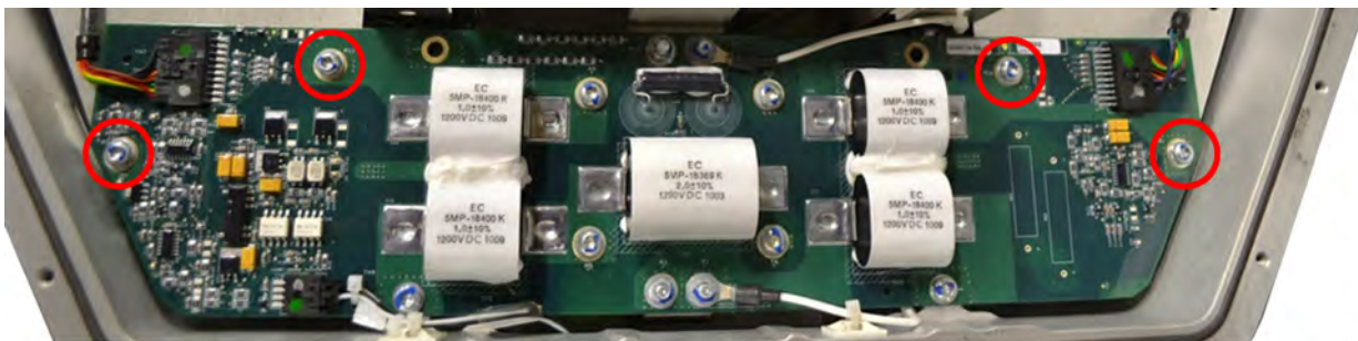
Figure 11. HVIL Circuit Card – Four (4) Mounting Screw Locations (M5x22mm)
