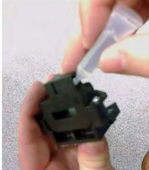
Figure 69. Applying NyoGel® 760G Synthetic Lubricant to Current Sensor Pins
