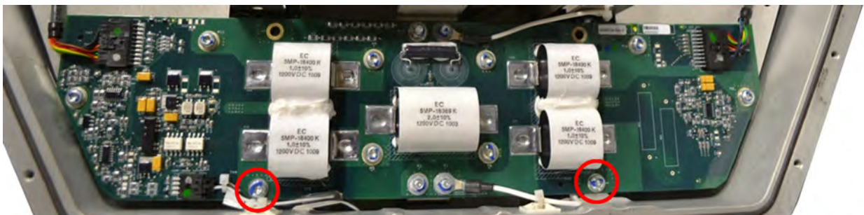
Figure 10. HVIL Circuit Card – Two (2) Mounting Screw Locations (M5x14mm)
