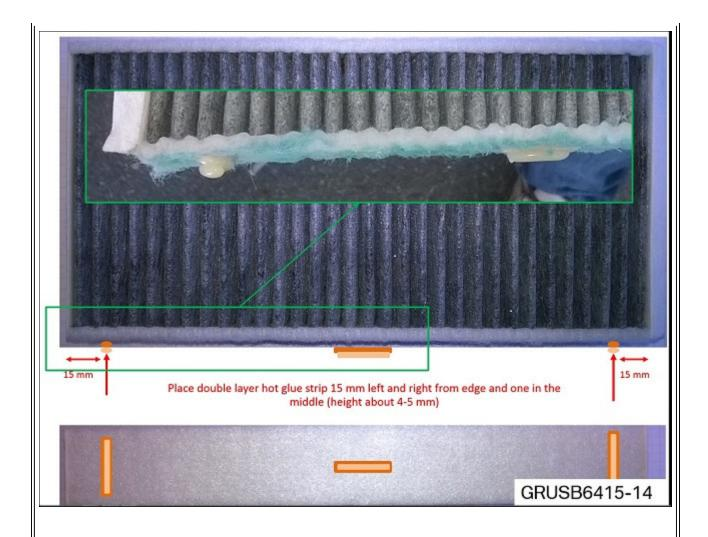
All 3 hot glue applications must be double layered, be 15 mm long and have a total height of 4-5 mm. Placement of the hot glue must be in the exact locations shown to prevent complications with condensate water flow.
