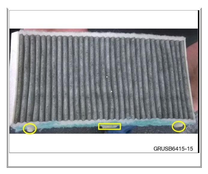
6. Allow the applied glue time to dry, then install the upper and lower micro-filters in the housing (REP 64 31 010).
