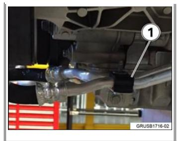
The cooler line block **should not** be mounted over the cooler line bracket (1). Relocate the plastic block under the bracket (tighten bolt to 10Nm).
