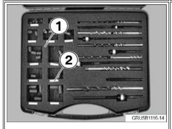
The special tool used to clean the threads is also found in the Helicoil Plus Thread Repair Kit P/N 81 43 A good quality M8 x 1.25 Spiral Fluted Tap can also be sourced locally to clean the threads.
