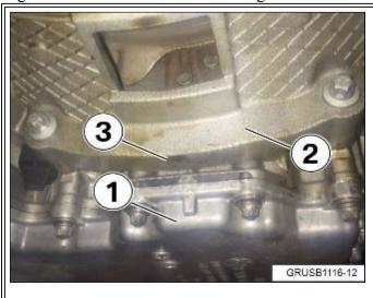
Engine oil pan (1) Transmission bell housing (2) Engine oil residue (3)
