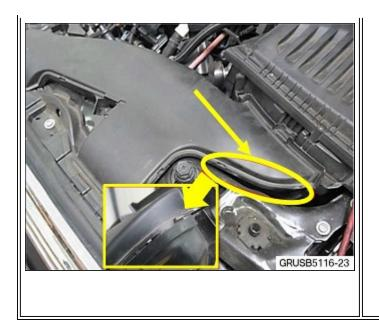
3. Inspect the intake air cover for consequential damage.The vibrations from a worn battery tray buffer can cause air intake damage in the area shown.
