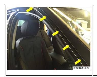
2. Use BMW Anti-Static cleaner (P/N 51 91 0 033 068), clean window guide contact areas to remove any residual wax or silicone.
