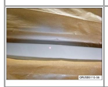
5. Mask off the area of the roof and clip for the roof frame trim strip and apply a preservative to the repaired area.
