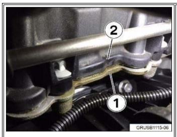
Engine oil leak (1) at the front edge of the cylinder head cover where it meets the cylinder head (2).
