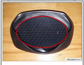
1. Lightly roughen the inner surface of the pedal cover with sandpaper. Clean out any remaining debris.
