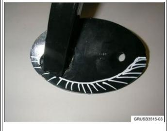
3. Apply Super Glue S1 to the rear of the brake pedal in the outlined area as well.
