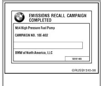
After the vehicle has been checked and corrected, obtain a label (SD 92-406) and with a ball point pen print your dealer code (5 digits) on the Recall Completion Label (see illustration). An initial quantity of 200 labels will be sent to all BMW centers. Peel the label from its backing and affix it to the right (passenger) rear side of the hood in the engine compartment, close to windshield.
