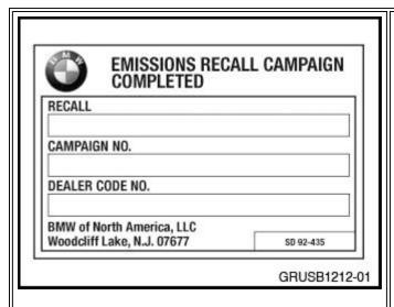
After the vehicle has been checked and corrected, obtain a label (SD 92-435) and with an indelible marker, legibly print the Recall name, Recall number, and dealer code (5 digits) on the Recall Completion Label (see illustration).
