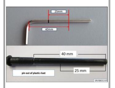
3. To remove the headlight ventilation filter, use a 3 mm Allen wrench.
