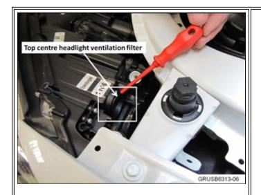
2. With a screw driver, remove the cap from the headlight as shown in picture.
