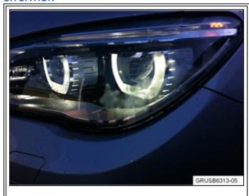
Condensation or fog forms inside the LED headlight lens cover
