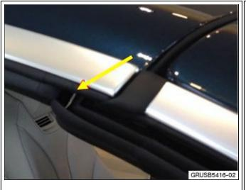
Photo at left shows gap between A-pillar seal and cowl panel seal (outside view).
