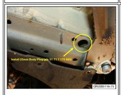
4. Install rubber body plug in location shown.
