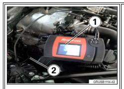
Use a bore scope (1) or similar (mirror) to help identify the injector index number on the injector (2).
