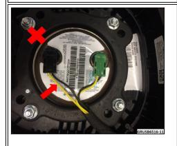
Incorrect routing. The yellow wire is under tension.
