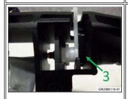
4. Make sure cable strap is secured and Bowden cable is seated securely as shown (in Figure 3).
